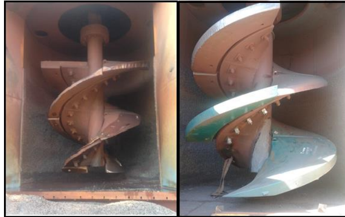
Figure 4 - Left: screw liner with intensive wear at the bottom. Right: new screw liner (Esteves et al., 2018).
